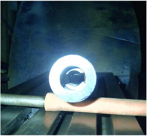
At this point your receiver blank should look like the picture above. Now I know what you are thinking I leave the receiver raceways square. The answer is NO I do not, when I am finished the raceways will have an arch very close to an actual Mauser receiver.
