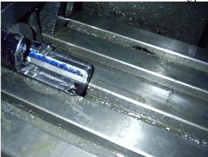
When ever you decide to cut the cocking piece groove this is how it will look. This picture also shows the rear tang reduced in height by approximately .060 inches, leaving the area directly under the bolt handle a the original height.
