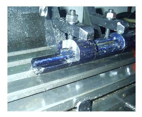
I now have one of two choices to make. I can either cut the groove for the cocking piece or go to the lathe and turn the eccentric notch for the safety lug. Since I know the length of the cocking piece groove to be 2.375 inches, I will go ahead and mill it now.
